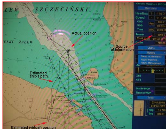
Fig. 6. Virtual movement of m/v Navigator XXI [own study]
