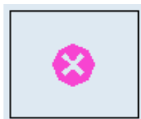
Fig. 3. Isolated danger of depth less than the safety contour: wrecks, obstructions, under water rocks [source: IHO publication S-52 Appendix 2 Addendum to Annex 2, Part I, Users' Manual Edition 3.4 2008]
