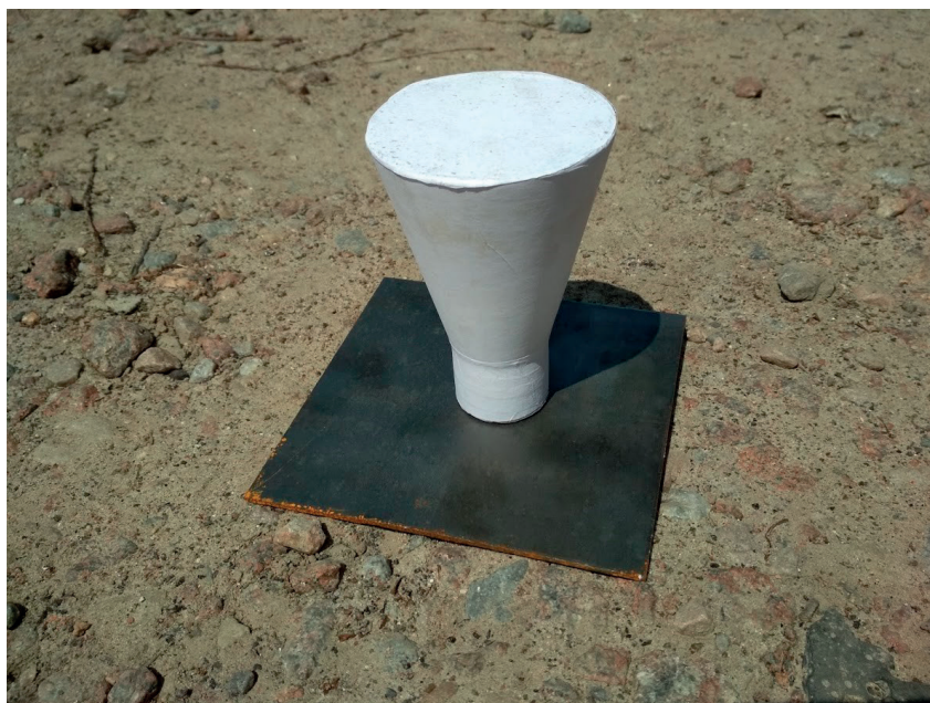
Fig. 5. An donor with a taper angle of 30° on a metal witnessplate
