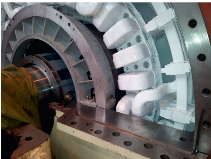
Photo 3. New rotor fan shield with rear guide vanes
