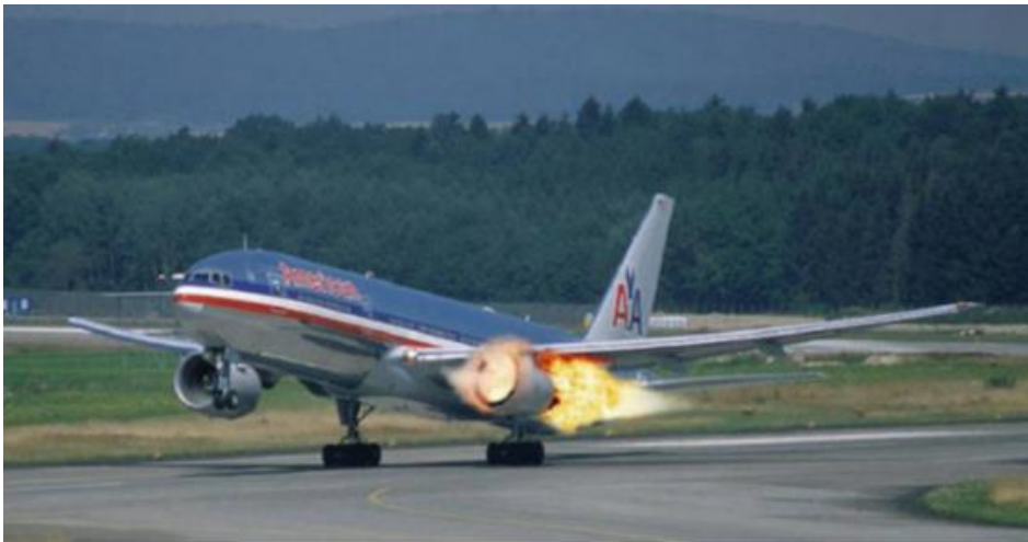
Fig. 1. Unstable compressor operation in a Boeing 777 leading to flame outburst [2]
