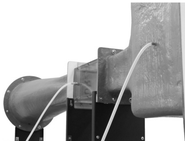
Fig. 3. Location of tubing connections
