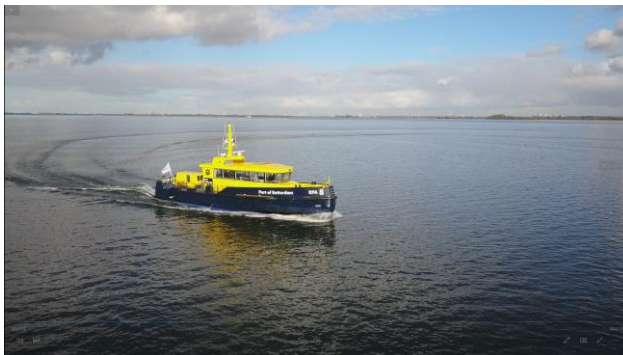
Fig. 11. RPA 8 has exceptionally low wavemaking properties and high efficiency [7]
