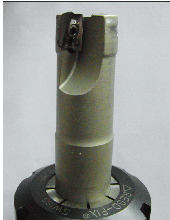
Fig. 2. End mill with diamond inserts
