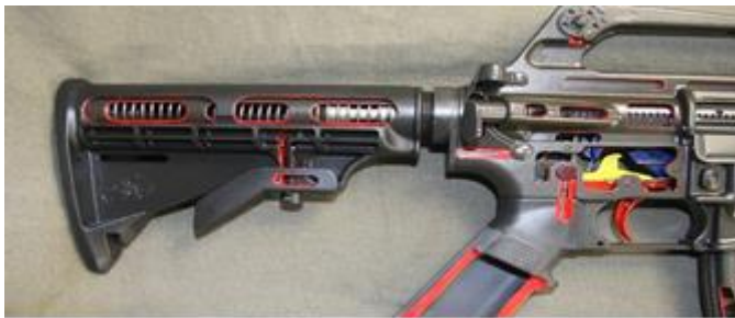
Fig. 8. Section of view of the 5.56 mm M16A1 assault rifle, the section clearly shows that the recoil mechanism is located in the stock [27]
