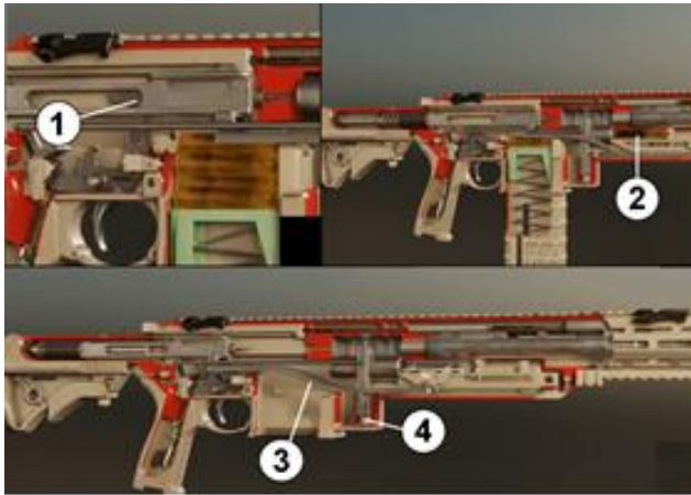
Fig. 4. Operation sequence of the 6.8 mm NGSW-R assault rifle prototype [15] 1 - Hammer, 2 - Extraction of the spent shell casing forward and to the side trough an opening in the lower front part of the weapon, 3 - Guide rails, 4 - Barrel springs
