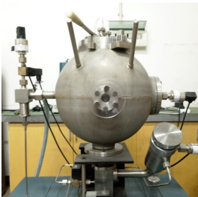
Figure 3. 20L explosion vessel experimental device
