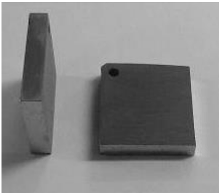
Fig. 1. Examples of the samples coated with nickel
