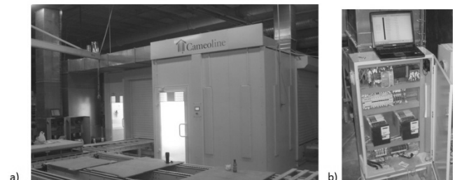
Fig. 6. A view of the real plant : a) the spray booth b) data acquisition from the control box
