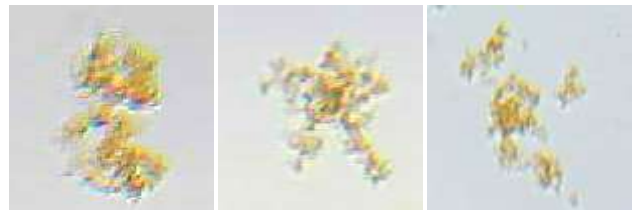
Fig. 4. Flocs without mass concentration
