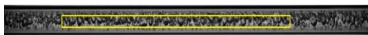
Fig. 3. A photo frame and the analysed area (rectangle) of water-glycerol and air flow: liquid flow rate ( q_w ) and air flow rate ( q_g ): q_w = 43,44 kg/h, q_g = 0,328 l/min [13].
