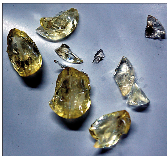
Fig. 10. Artificial amber after pulsed power plasma discharge in silicone oil (single shot)
