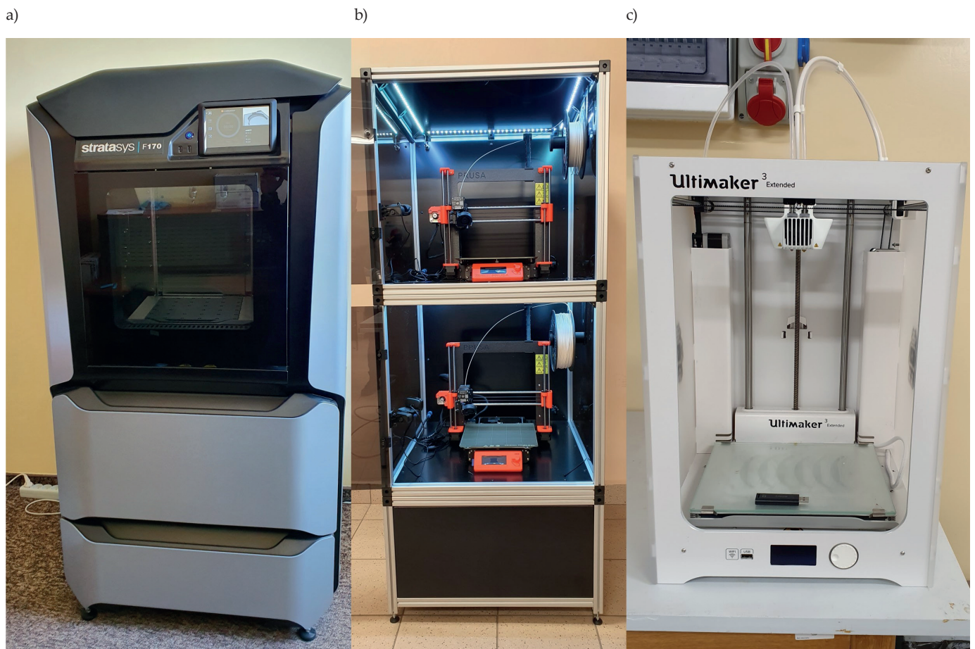
Fig. 2. Devices working in the technology of layer extrusion of thermoplastic polymers: a) Stratasys F170 printer, b) a set of integrated Prusa printers, c) Ultimaker printer
