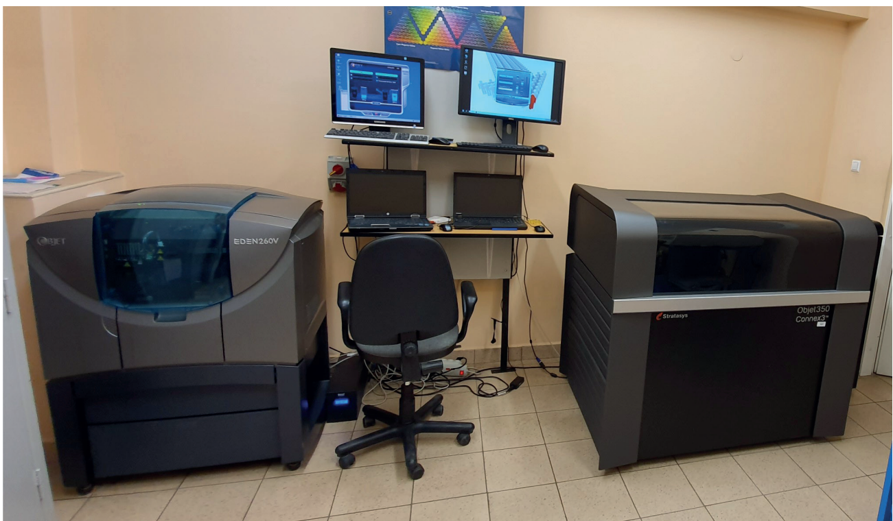
Fig. 1. Objet Eden 260 and Objet 350 Connex 3 3D printers connected to the control computers by the network
