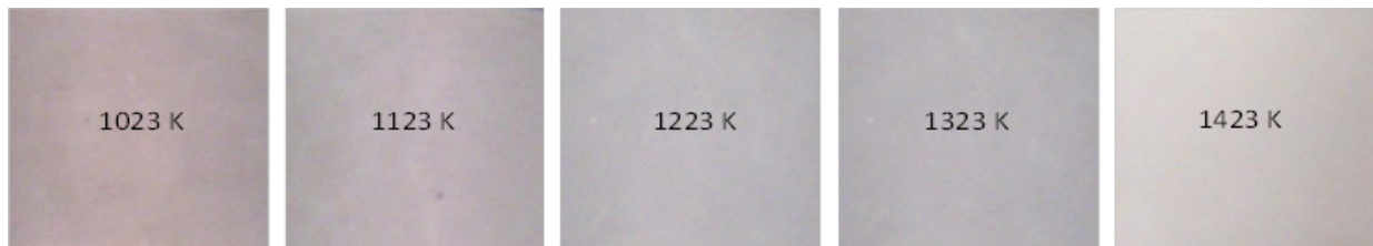
Fig. 1. Images of sample surface from the turbine rotor blade heated at different temperature [4]
