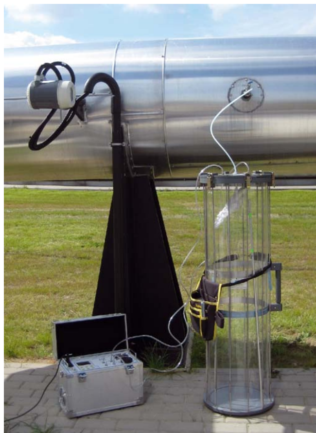
Figure 4. Sampling for the determination of odour concentration
