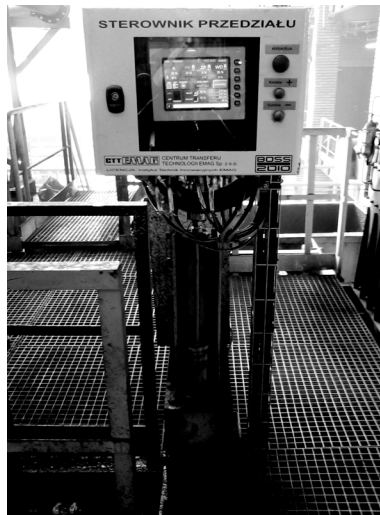
Fig. 5 Computer-controlled EMAG-type system BOSS2010 in LW BOGDANKA [14]
