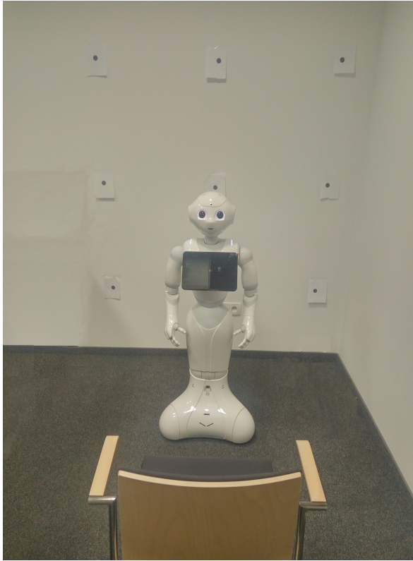
Figure 5. Test environment – robot and direction markers
