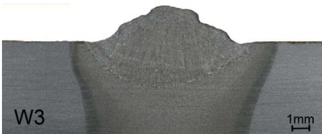
Fig. 3. Macro cross-section of the welded specimens W1, W2 i W3 (specimen without insulation W). Etch. Nital
