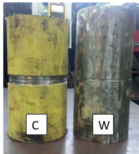
Fig. 1. Specimens prepared to welding. C – specimen covered with anticorrosive polymer coating; W – specimen without the coating.
