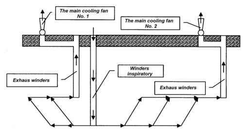
Fig. 1. A model diagram of ventilation network A
