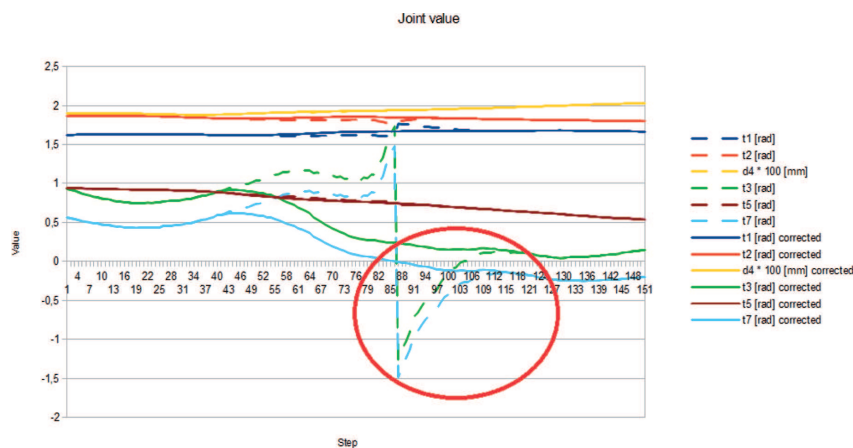
Fig. 9. Desired (a dotted line) and reached as the result of the safety function (a continuous line) joint variables, while passing a singularity
