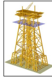
Figure 2. Offshore template (jacket) platform [10]
