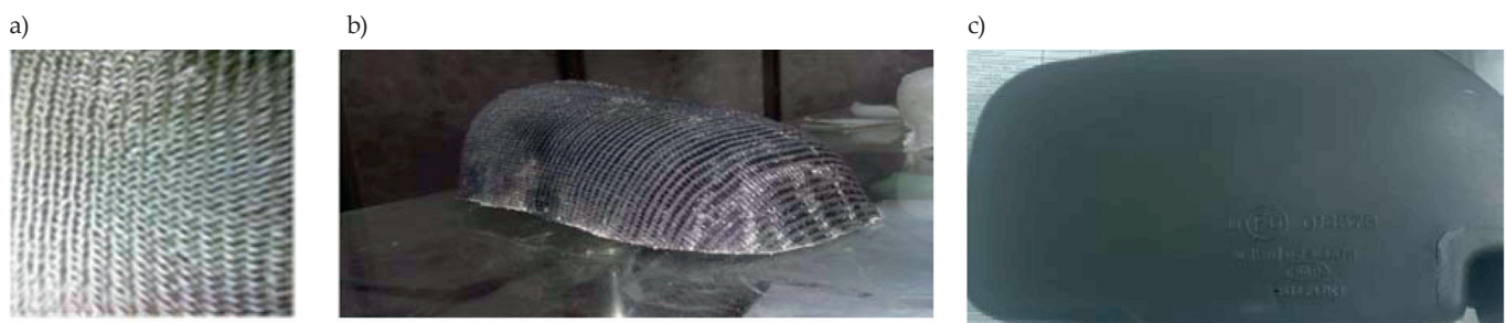
Fig. 2. Composite and market samples: a) knitted sample, b) basalt knitted composite, c) market sample
