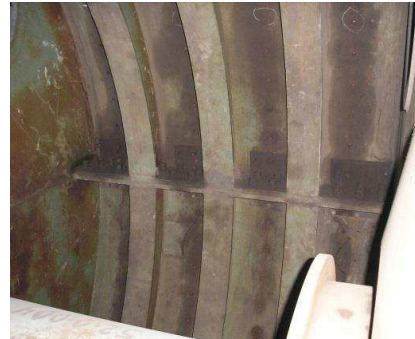
b) shell with circumferential ribs
