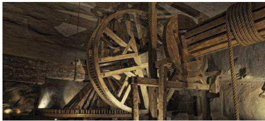
Fig. 3. Horse gear Wieliczka Salt Mine [1]
