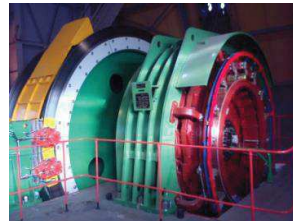
Fig. 2. Two-rope hoisting machine of Koepe type
