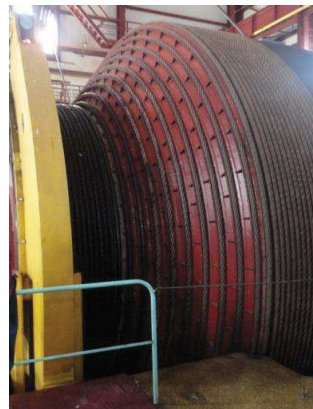
Fig. 6. Cylindrical-conical winding drum with direct grooving on the drum shell
