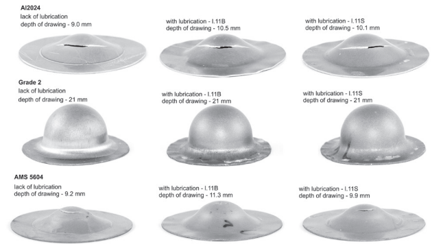
Fig. 3. Effect of lubrication on spherical cap drawing process
