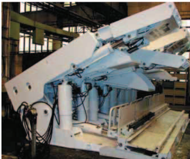
Rys. 8. Obudowa zmechanizowana BMV – 1Mi [5] Fig. 8. Hydraulic powered support BMV – 1Mi [5]
