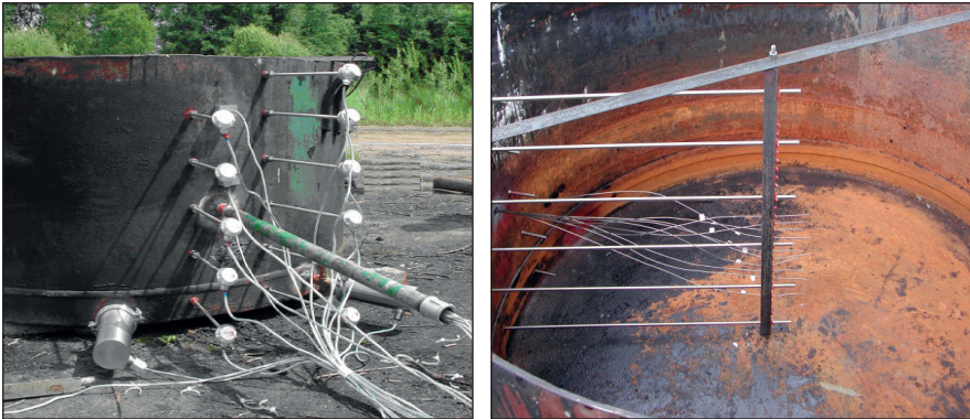
Fig. 3. Location of thermocouples in the tank 70 cm high
