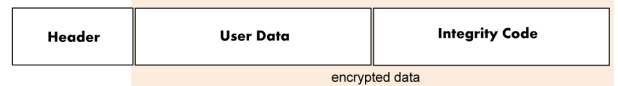
Fig. 2. The structure of information in safe transmission systems according to norm PN-EN 50159:2011 [13]
