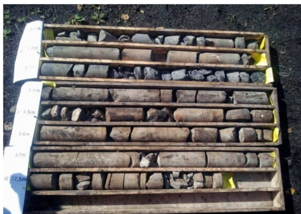
Fig. 5. Typical view of a core log from the borehole.
