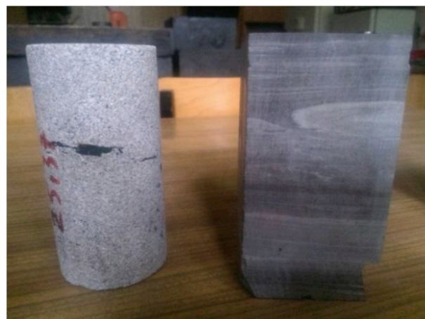
Fig. 3. The sandstone specimen with coal lamina (cylindrical) and the claystone specimen with quartz laminae (cuboid).
