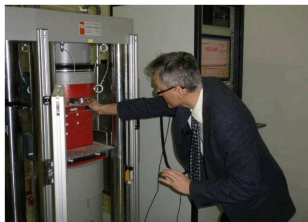
Fig. 4. The compressive strength test on claystone on Walter + Bai servo-operated press.
