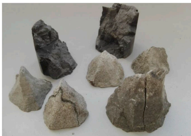
Fig. 6. Typical conical shape of rock samples after their damage.
