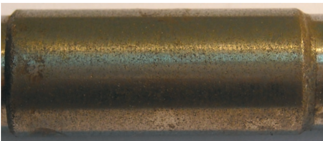
Fig. 12. Molybdenized shaft surface after fatigue tests – no fretting wear; magnified about 3x
