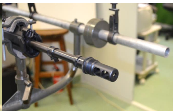
Fot. 4.6. Karabinek systemu MSBS-5,56 z UW-5 na stanowisku badawczym Photo 4.6. Carbine of MSBS-5.56 system with MD-5 on the set-up
