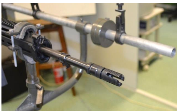
Fot. 4.5. Karabinek systemu MSBS-5,56 z UW-4 na stanowisku badawczym Photo 4.5. Carbine of MSBS-5.56 system with MD-4 on the set-up
