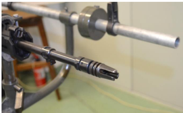
Fot. 4.3. Karabinek systemu MSBS-5,56 z UW-2 na stanowisku badawczym Photo 4.3. Carbine of MSBS-5.56 system with MD-2 on the set-up
