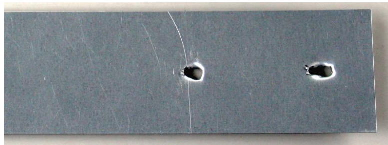
Fig. 3. Example of a connection bearing failure
