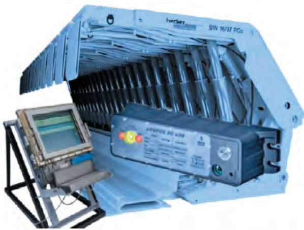
Fig. 6. The active pressure maintenance system from Elsta [22]
