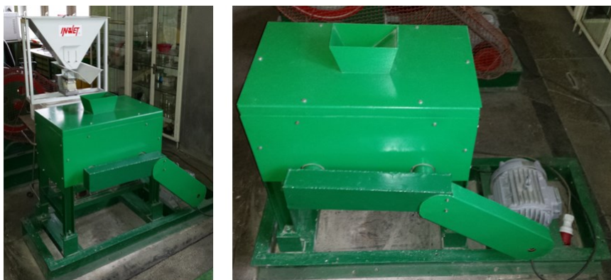
Fig. 6 KWB-d vibratory jaw crusher with lower jaw suspension located in the AGH Department of Mining, Dressing and Transport Machines laboratory
