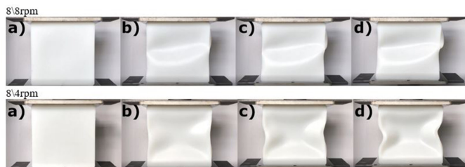
Fig. 9. Compression test conducted on parts moulded with speed ratios of 8\8 and 8\4 rpm, where: a) test piece at the start of the test, b) test piece after 10 s of testing, c) test piece after 15 s of testing, d) part after the compression test
