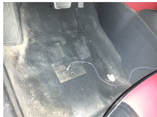
Fig. 2. Accelerometer positions on vehicle floor.
