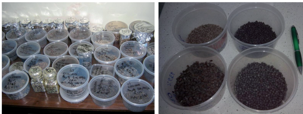
Figure 3. Ready for hot tests manganese oxides ceramic based catalysts in the form of pellets (some of them doped and/or promoted) [Aut., 2015]
