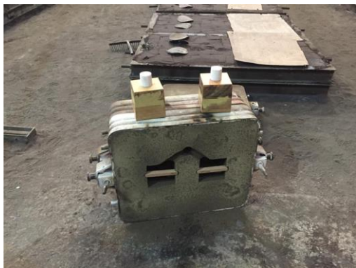
Fig. 4. The cope, prepared for steel iron casting
