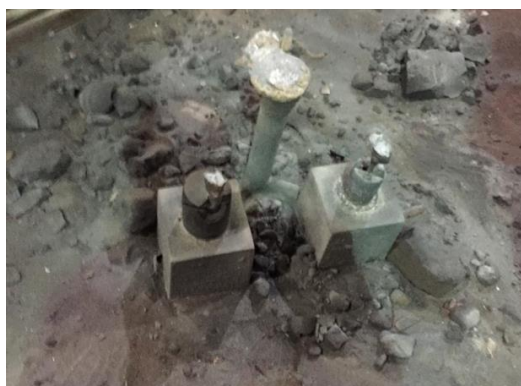
Fig. 5. Cooled steel parts after shake out
