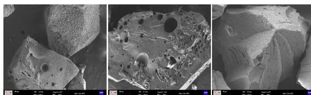
Fig. 8. Images of DBE cured resins from 100 microns, left to right, respectively; Standard Alfanol (294X, 5kV, 5.9 mm), Lignin mod. (298X, 7kV, 6.7 mm) and Resorcinol Mod. (500X, 5kV, 6.6 mm)
