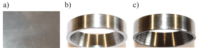
Fig. 2. Materials for abrasive wear tests a) Aluminium alloy 2024 strip, b) Counter sample of NC6 steel, c) Counter sample of WCL steel
