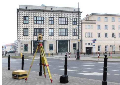
Fig. 3. The station during measurements of the building's facade of the Warsaw Ballet School
