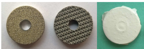
FIG. 1. Representative images of plasma treated and printed titanium samples before and after application of collagen/antibiotic layer (right).
