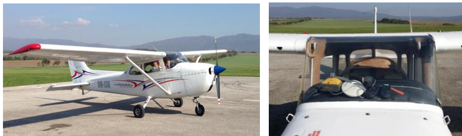
Fig. 6. Cessna plane taking part in the experiment and location of GNSS antenna
