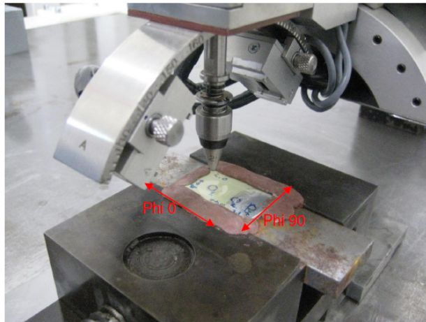
Photo 3. Plate with three different areas. Directions of measured stresses.
