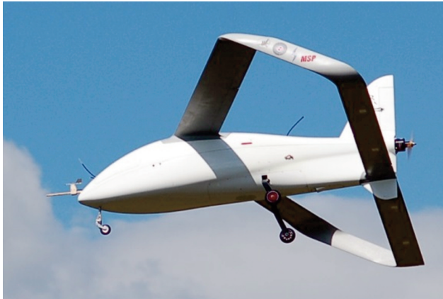
Fig. 1. Original configuration of ILX-32 MOSUPS.
