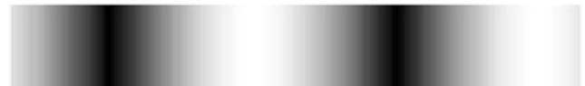
Fig. 3. The 2-D image of a pure sinusoidal waveform with 32 cycles and the cycle length exactly equivalent to the period
