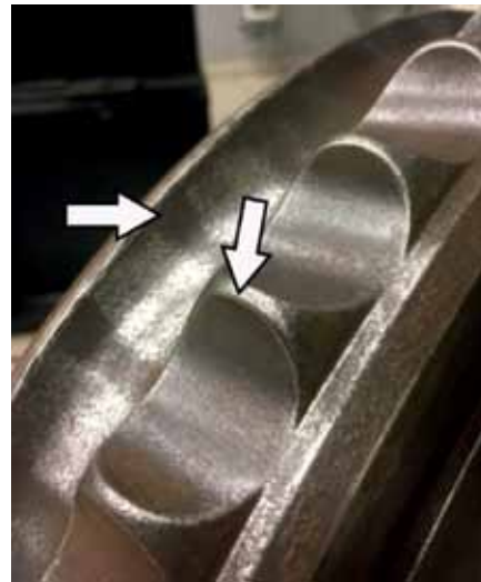
Fig. 6. Operating wear mechanism of conventional moulding rings used for the production of saddle-shaped briquettes
