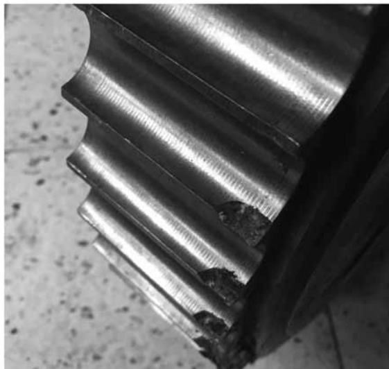
Fig. 10. View of the part of the working surface of the system that is the subject matter of patent application No. P-393053 that has been destroyed as a result of a test drive operation of only one roller of the briquetting machine
