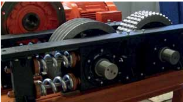
Fig. 5. Scheme of an asymmetric compaction unit where the sides of the profile of consecutive rows of cavities is not swapped [27]
