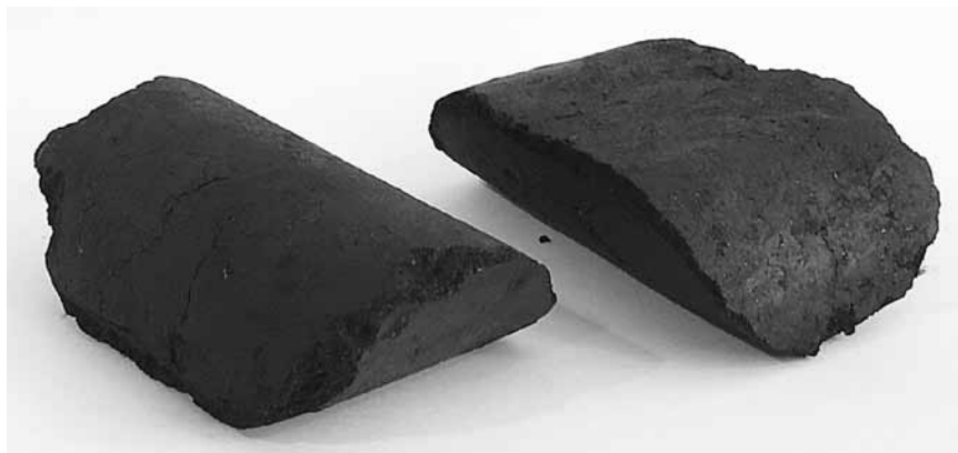
Fig. 8. Saddle-shaped briquette with its volume increased through the extension of one of its sides lying along the moulding ring generatrix
