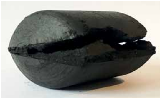
Fig. 1. View of a briquette consolidated in a roll press with a symmetrical compaction unit and delaminated along the parting plane
