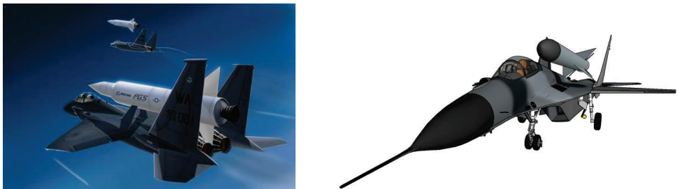
Fig. 1. Air-assisted rocket systems: on the left Boeing concept [6] and the right MUT version [7-12]
