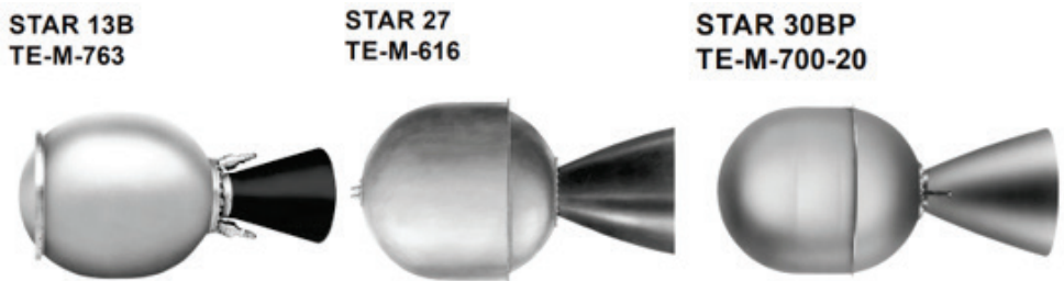
Fig. 12. The motor models used in the three-stage rocket concept [24]
