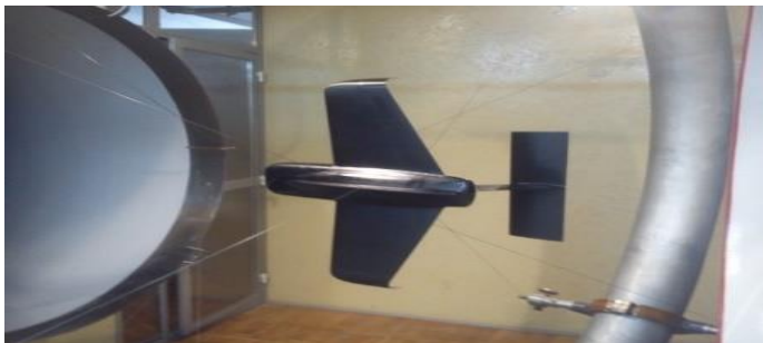
Fig. 4. Actual model suspended in the wind tunnel [9]
