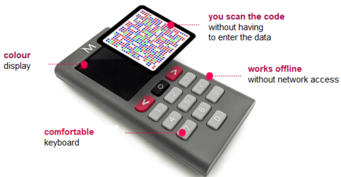
Fig. 10 - Hardware token from Millennium Bank [13]
